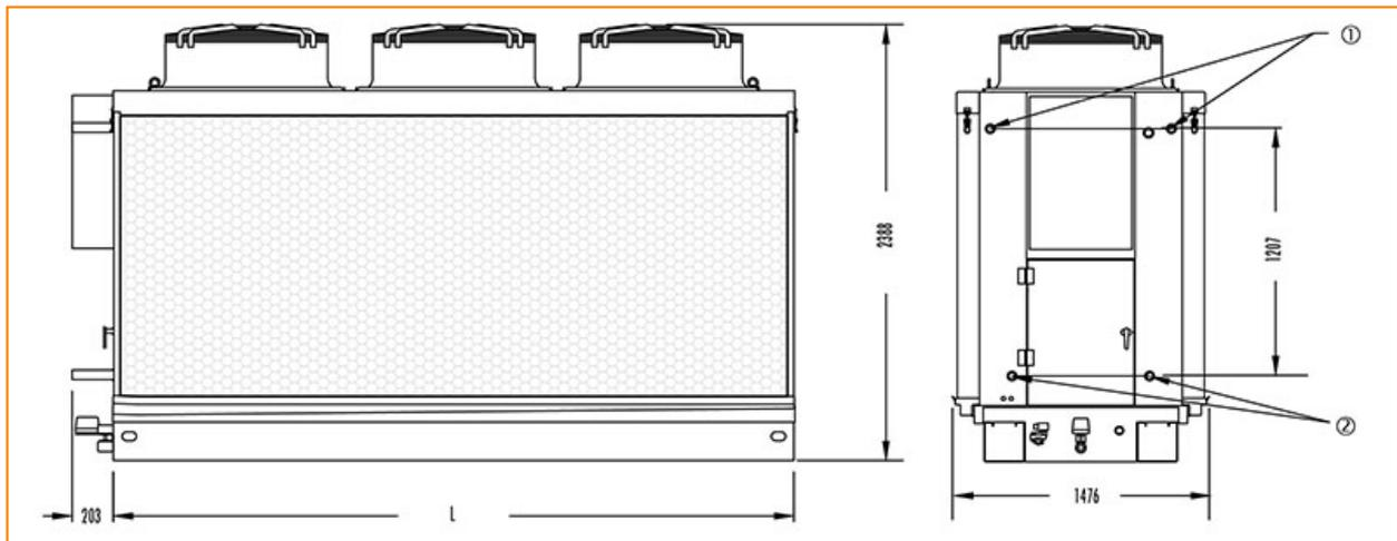
1. Refrigerant inlet connections; 2. Refrigerant outlet connections. TSDC-CO2-044-3
