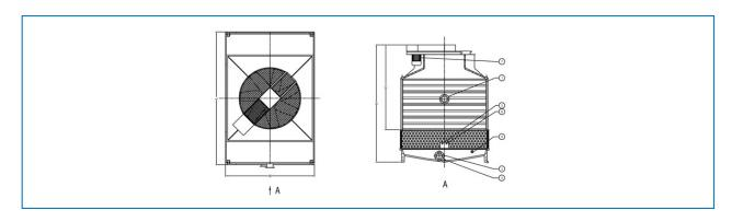
1. Water inlet; 2. Water outlet; 3. Drain; 4. Overflow; 5. Make up; 6. Quick fill; 7. Fan motor.
