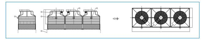
1. Water inlet; 2. Fan motor; 3. Concrete basin (by others).
