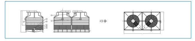
1. Water inlet; 2. Water outlet; 3. Drain; 4. Overflow; 5. Make up; 6. Quick fill; 7. Fan motor.
