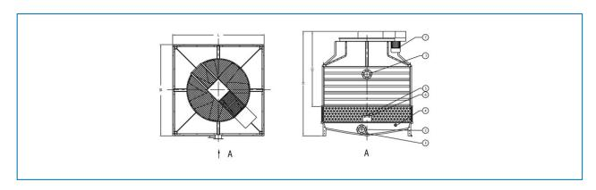
1. Water inlet; 2. Water outlet; 3. Drain; 4. Overflow; 5. Make up; 6. Quick fill; 7. Fan motor.
