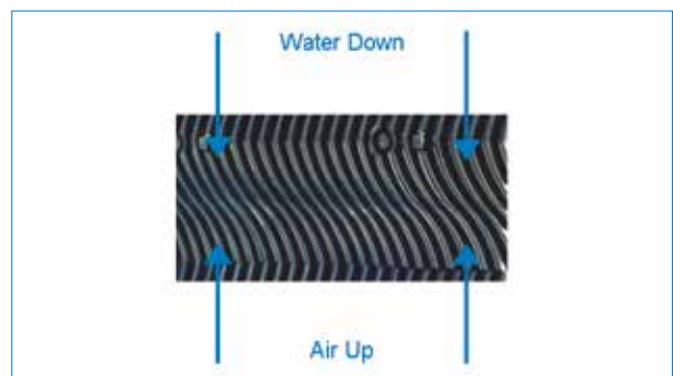
Counterflow Configuration (open cooling towers)
