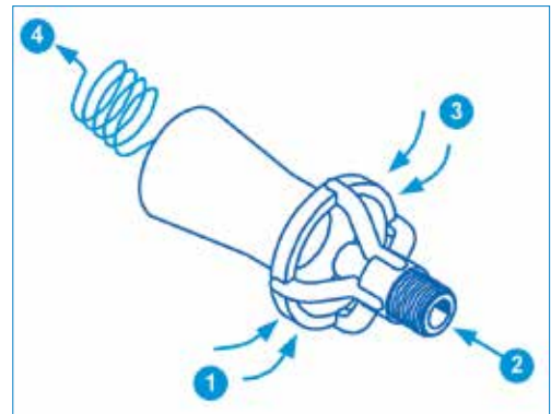
Figure 5: Eductor 1. Sweeping: Circulate four Litres of Sump Water; 2. One Litre of Filtered Water from Pressure Line; 3. Eductor; 4. Five Litres Circulated
