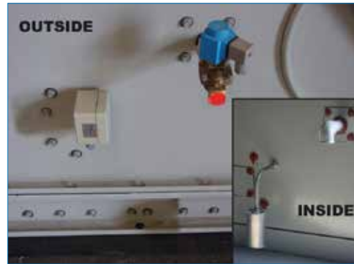
Electronic Water Level Control
