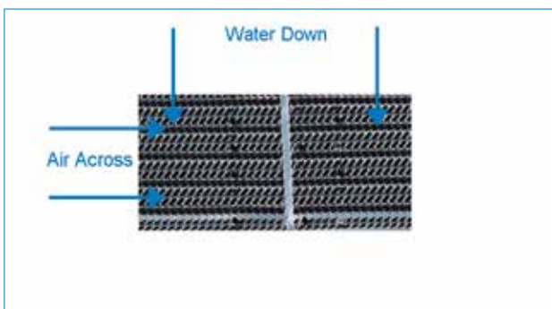
Crossflow Configuration (open cooling towers only)
