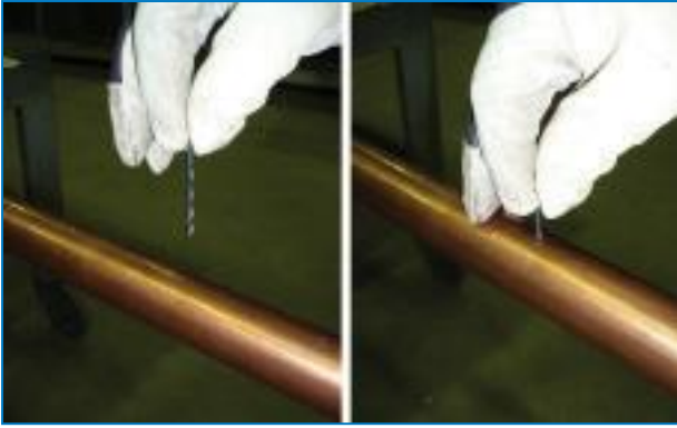
Clean Spraying Holes
