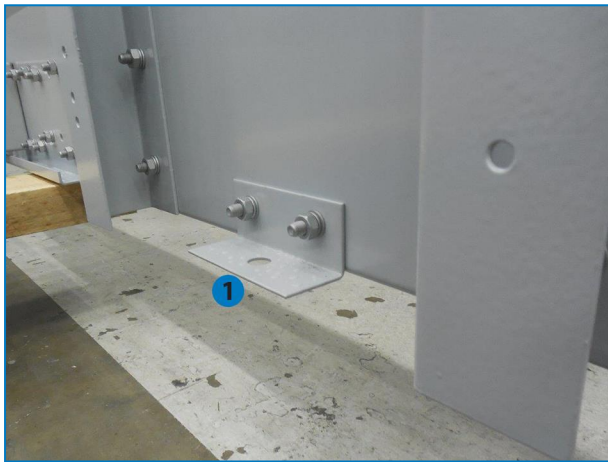
1. Rigging guide/bracket of upper section
