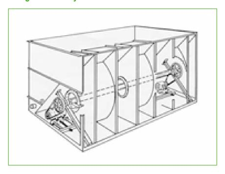
The installation of a Baltiguard® drive system
