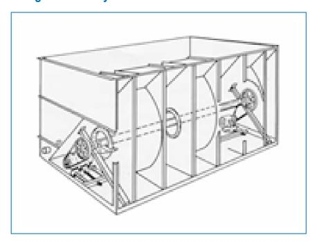
The installation of a Baltiguard® Drive System
