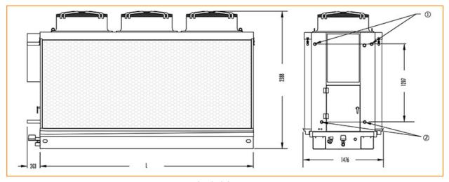
1. Refrigerant inlet connections; 2. Refrigerant outlet connections. TSDC-CO2-044-3
